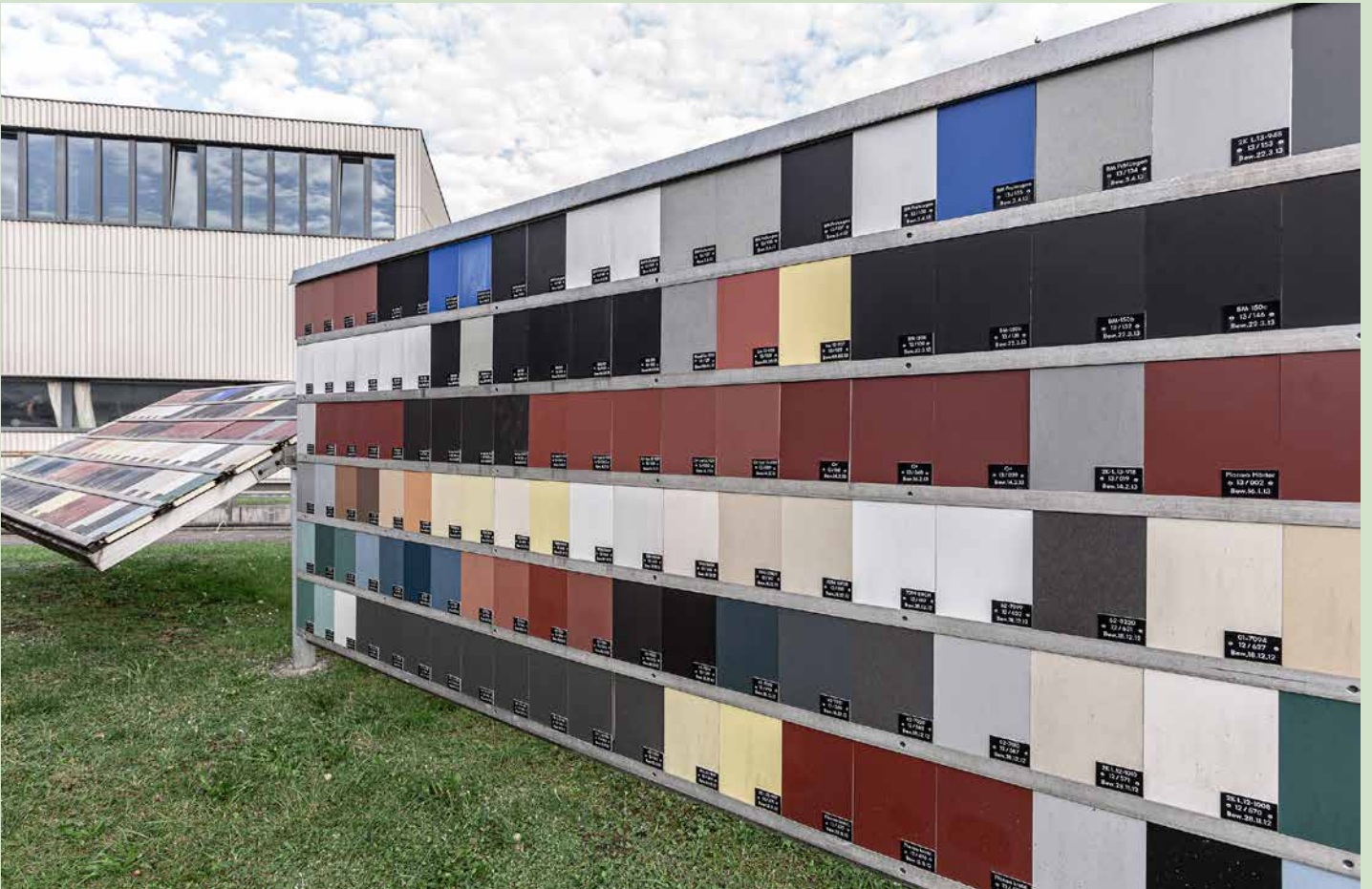
The outdoor weathering unit tests the steadfastness of the coatings in real-life conditions over a period of years.
