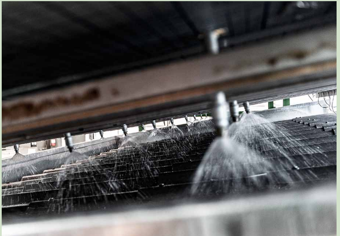
The panel prototypes undergo further material stress tests using the rain machine.
