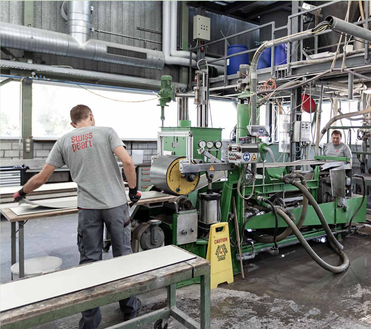
The Mini Hatschek machine creates test-size prototypes with all the qualities of the full-size product.
