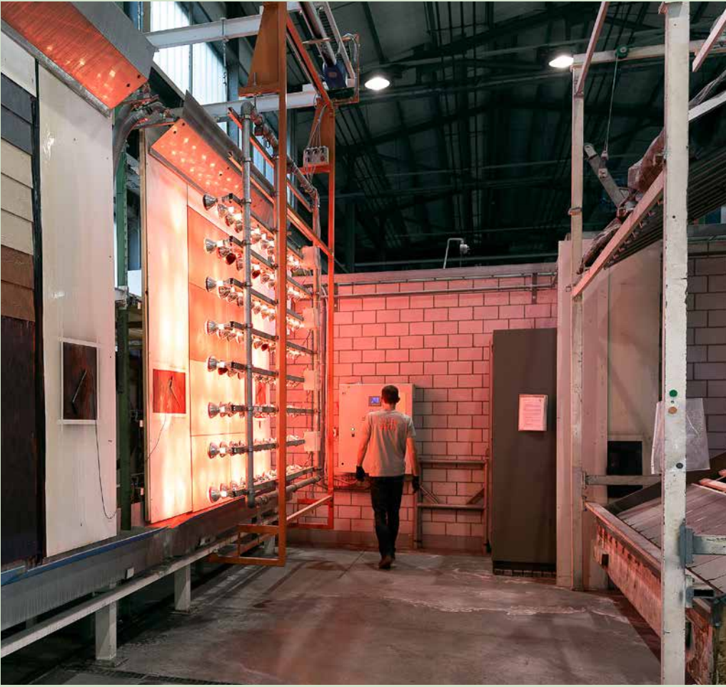
The heat-rain test simulates extreme climate conditions with high temperatures and heavy precipitation.
