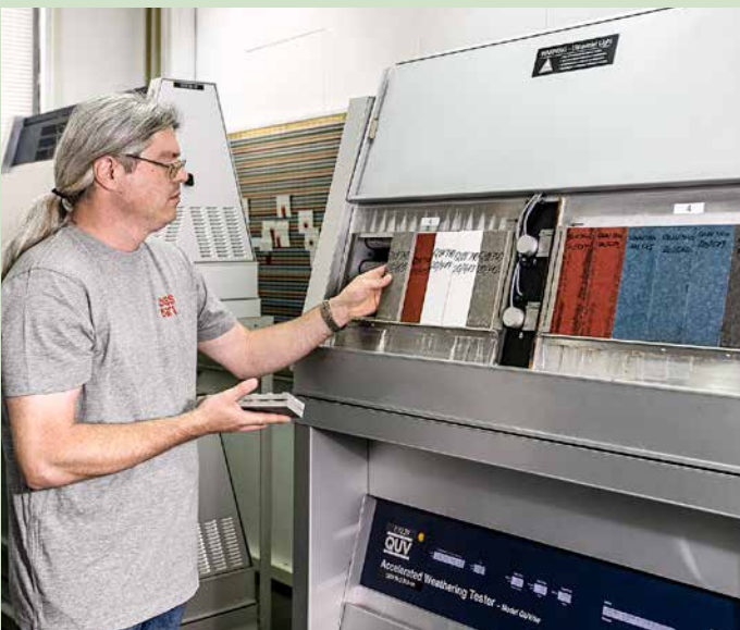
In the laboratory, the color coatings undergo UV resistance tests.
